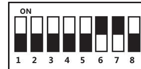
DIP Switch of Wiegand 26 Protocol
